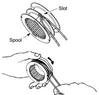
With your finger between the lines, wrap the lines evenly and firmly around the spool in a clockwise direction.8. Position the lines in the guide slots.
